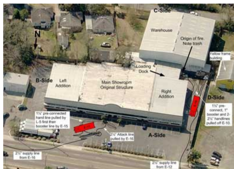
Diagram 2. Location of Engine 10 and Engine 11, supply lines and hose lines pulled at different times during the incident. Note accumulation of trash at loading dock on the day photo was taken, 3 months prior to the incident. Note the absence of ventilation ductworks or other roof penetrations over the showroom, thus no path for smoke and hot gases to escape.
