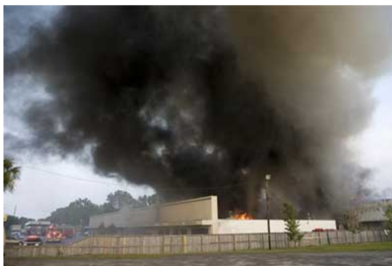
Photo 2. Time approximately 1930 hours. Note how smoke has changed to dark black color indicating it is rich with products of incomplete combustion. Note Ladder 5 and Engine 11 in front of structure as well as fire department vehicle in lower left corner. The top of Engine 10 is just visible over the fence at the lower right.
